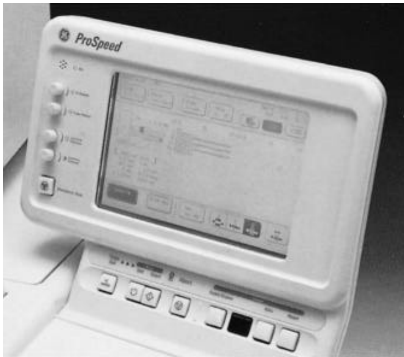
Simultaneity functions of Scan, reconstruction, Image Display and Analysis are controlled from the Operator Console
